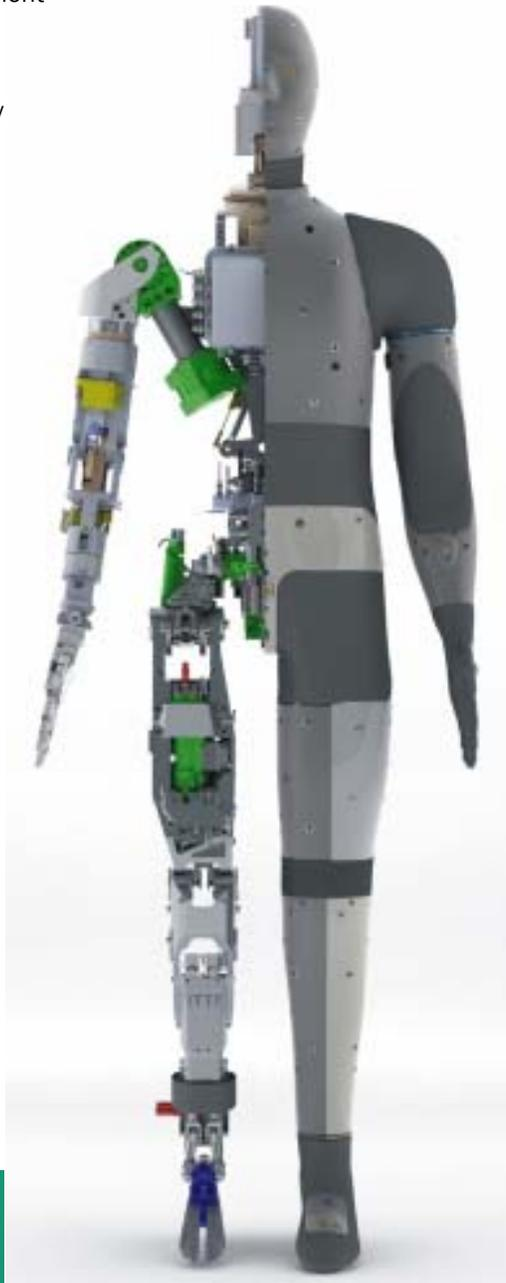
A prototype leg was also designed and built in 2009 to prove the efficacy of Measurement Technology NW's proposed thermal and perspiration systems, while also serving as a vehicle for chemical test exposure to help gauge raw material performance (absorption rates, decontamination requirements) as well as the flexibility and effectiveness of joint seals.
