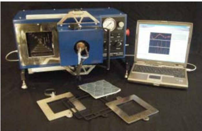
MTNW's Stored Energy Test Device includes a radiant heat source, specimen holder, sensor assembly, transfer tray with water-cooled carriage, pneumatically-actuated compressor assembly, data acquisition/control system, and PC with burn damage analysis software.
