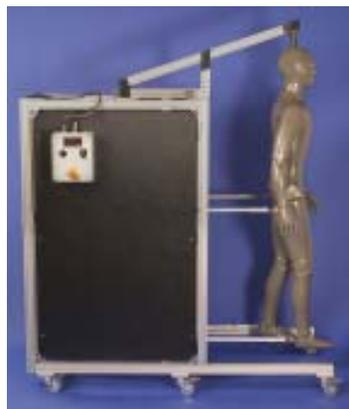
MTNW engineers have redesigned the Newton Motorized Walking Motion Stand as a more compact unit that's easier to move through low doorways and tight spaces. Newton's up-front mounting point maintains the integrity of ambient airflow around the manikin. Mounting is now accomplished via an integrated head post for minimal interference and easier manikin dressing.
