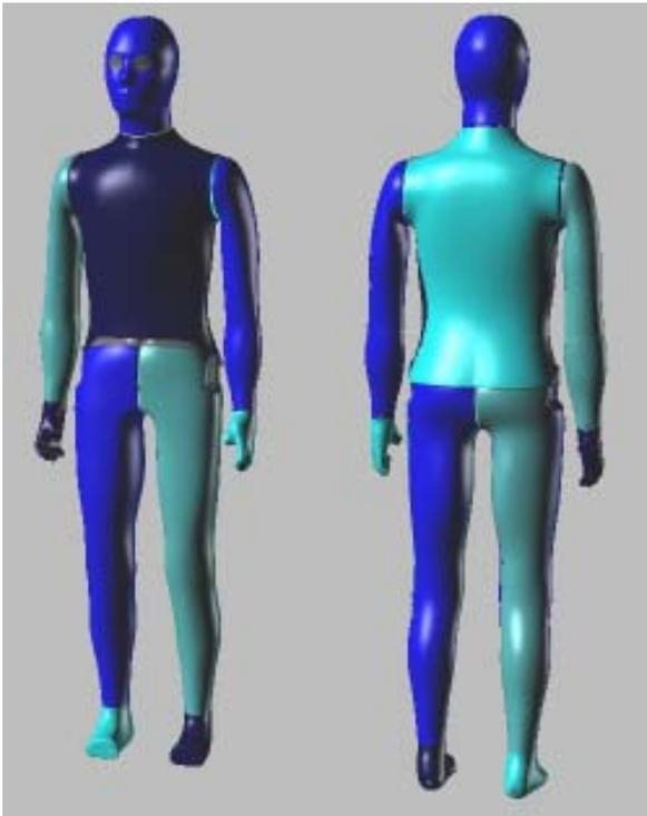
As shown in the CAD model images above, the 13-zone Simon format includes independent thermal zones at the Head, Torso (front/back), Arm (left/right), Hand (left/right), Leg (Front left/right, Back left/right), and Foot (left/right). This design helps maximize production efficiencies while yielding a thermal manikin that retains all of the advanced measurement and control features that have made MTNW systems the most popular thermal manikins available today.
