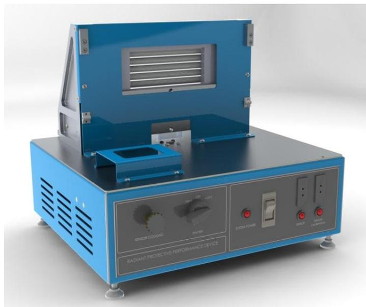
materials being tested and reaches the sensor, the temperature rise is depicted as a curved line that is automatically compared to Stoll's curve, which represents the blister point of human skin as a function of heat and time. The point of intersection between the test's curve and the Stoll curve provides a fabric's RPP/RHP rating.
